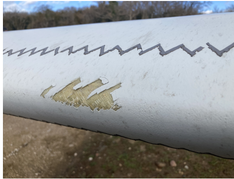
Figure 1: Wind turbine blade with LEE
